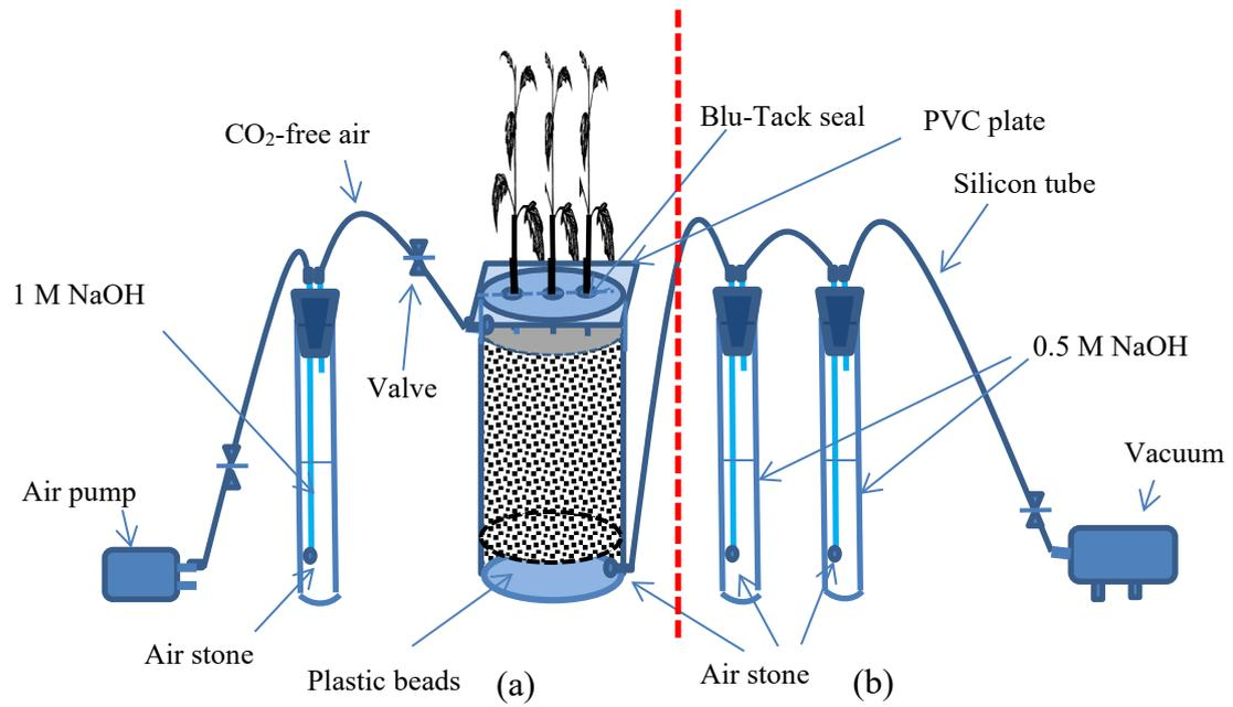
**Figure 1.** Trapping system of CO<sub>2</sub> released from belowground [(a): leak checking; (a) & (b): CO<sub>2</sub> trapping] (Modified from Cheng *et al.* (2003)).
