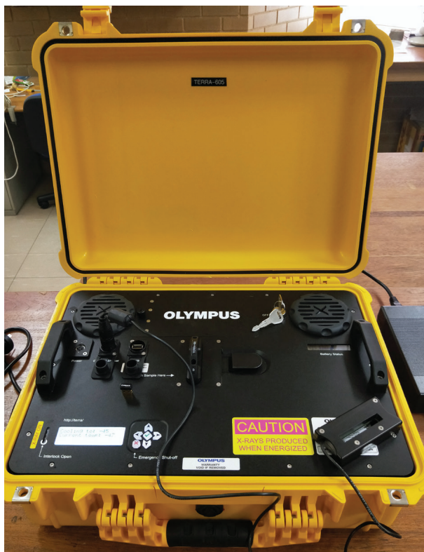
Figure 1. The Olympus TERRA portable XRD analyser and the ‘shaker’
